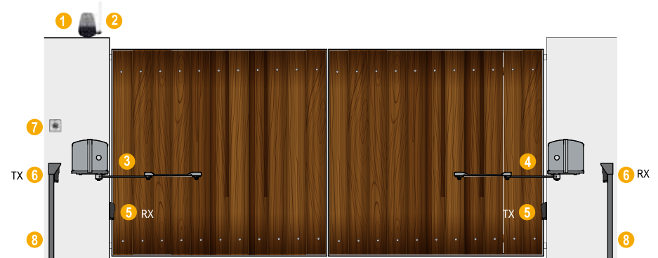
1_Flashing light 2_Outstanding antenna 3_LH operator featuring control board and radio receiver 4_RH operator Motoriduttore destro 5_Outer photocell 6_Inner photocell 7_Key switch 8_Photocell posts
