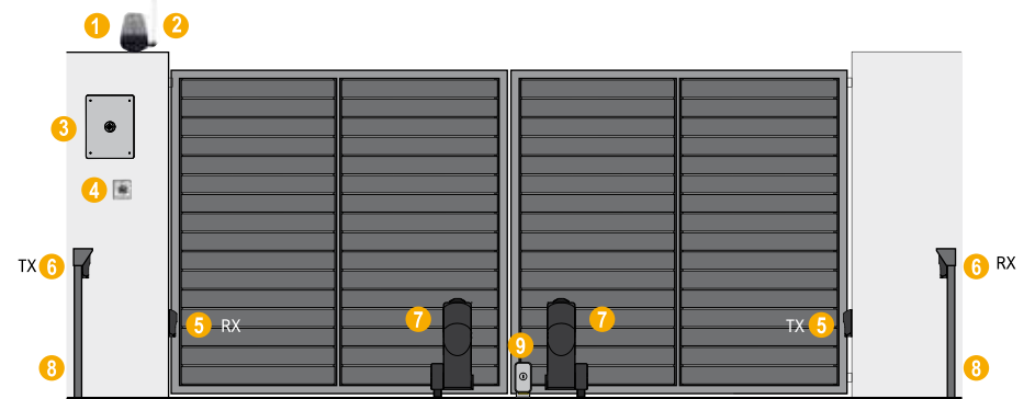
1_Flashing light 2_Outstanding antenna 3_Control board 4_Key switch 5_Outer photocell 6_Inner photocell 7_Wheel motors 8_Photocell posts 9_Electric lock
