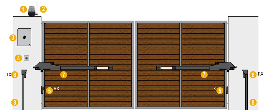
1_Flashing light 2_Outstanding antenna 3_Control board 4_Key switch 5_Outer photocell 6_Inner photocell 7_Swing operators 8_Photocell posts
