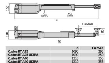
Complete range of electromechanical pistons for residential use, suitable for swing gate leaves up to 4 metres wide and weighing up to 500 kg. Quick and practical installation: the new KUSTOS BT A operators are designed to allow a quick and easy installation thanks to a numbers of important measures such as the magnetic limit switches and the magnetic locking pin.
